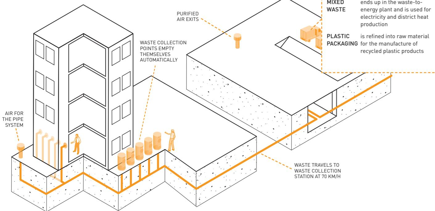
**THE NEW** era of residential living calls for brand new recycling solutions. At Jätkäsaari, there is a new, innovative pipeline-based waste collection system which introduces hi-tech into waste management on an unprecedented scale. Using an underground pipe network, waste travels to the waste collection station in a flash. Trucks gather the waste and transport it onwards – waste is utilized as recycled material, incinerated for energy or converted into biogas.
